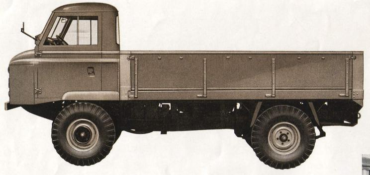
The Forward Control Land-Rover is primarily a load carrier and is available with various types of body suitable for the carriage of bulk loads and personnel. It can be supplied with a flat platform, a fixed-side body, or a drop-side body (left). A truck cab is standard equipment, but rear seats and hoods are also available.
